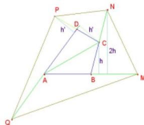
$$\begin{aligned} [BMN] &= 2[ABC] \\ [PQD] &= 2[ACD] \\ [BMN] + [PQD] &= 2[ABCD] \end{aligned}$$
